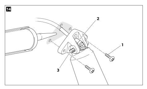
➤ When the bracket is fixed to the hull, remove the pivot bolt (fig 14 item 3) and lower the actuator to create clearance for the final screw, taking care not to pull the actuator harness out of the hull. Install the final screw, again taking care not to over-tighten. Reinstall pivot bolt, including the washer provided beneath the nut. Tighten nut to 30–40 in-lbs. Take care not to over-tighten.
