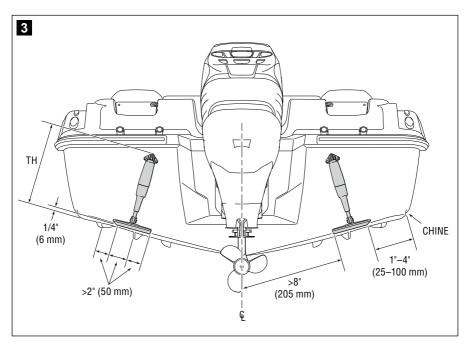
There are different tab configurations available and they will have different transom height (TH) requirements as shown in figure 4. The actual transom height will vary with the angle of the transom, so the maximum value for TH is shown.
