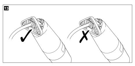
Insert the harness into the hole in the hull and feed it through until the actuator bracket is almost at the hull.
